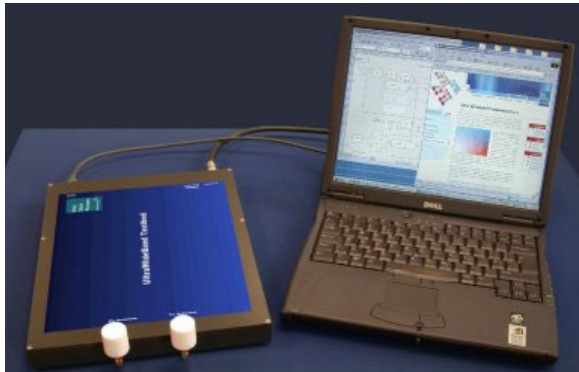
Figure 1: RMR UWB Hardware
