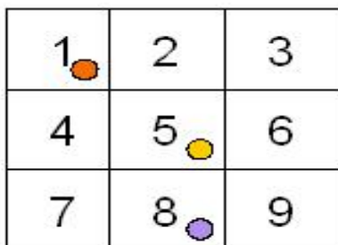
Figure 5: Event Addressing, pixels accessed in order events occur 5, 1, 8.
