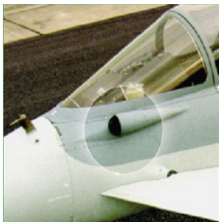
Figure 4: A single-aperture optical system mounted on an aircraft. Such components could be deployed around the aircraft in order to create an OAS array
