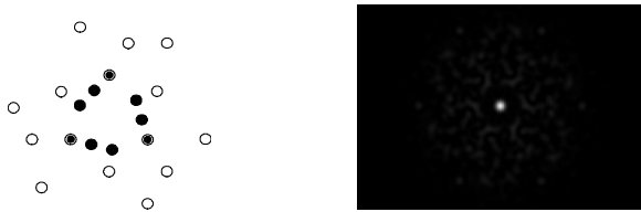
Figure 1: Schematic of a self-calibrating OAS system and the resulting snapshot PSF. Redundant Spacings Calibration (RSC) provides self-calibrated data from which diffraction-limited snapshot imaging can be achieved. On the right a single collector PSF would fill the picture (low-level sidelobes, not easily seen above, extend to the edge of the image). The central spot is slightly 'superresolved' - the sidelobes are a penalty paid for enhanced resolution. This 21-aperture arrangement is probably too complex for military applications, but shows what can be achieved through OAS.
