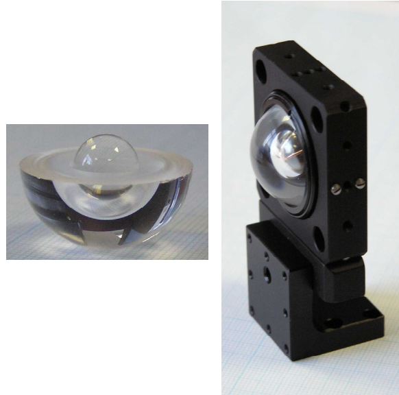
Practical GRIN-sphere: Partially assembled lens (left); Complete, mounted assembly with spacer (right)
