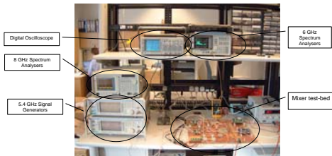
Figure 14: RMRL's FRM test-bed experimental set-up
