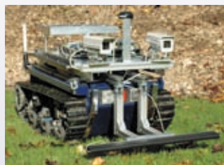
Roke's vision system has been integrated with experimental platforms to exercise the vision algorithms. The chassis of this vehicle has been loaned by Dstl.
