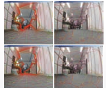
Local adjustments to triangulation can provide much improved estimates of scene structure. Here the output provided by the raw Delaunay triangulation (top images) misinterprets the floor. Adjusting the triangulation of a single group of features provides a faithful representation of the floor (bottom images).
