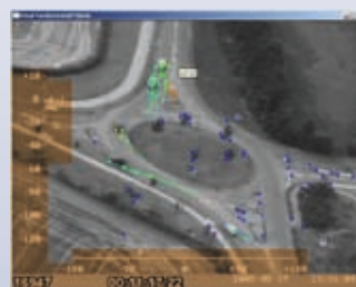
Stage 2: A 2nd classification of targets is obtained by analysing initial classification histories to identify a high-confidence stationary set (small blue crosses). This set is used for a further iteration of fundamental matrix calculation and consistency analysis.
