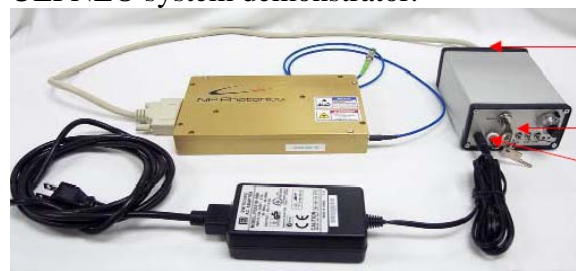
Figure 2 – 1kHz linewidth 1550 nm single frequency laser
