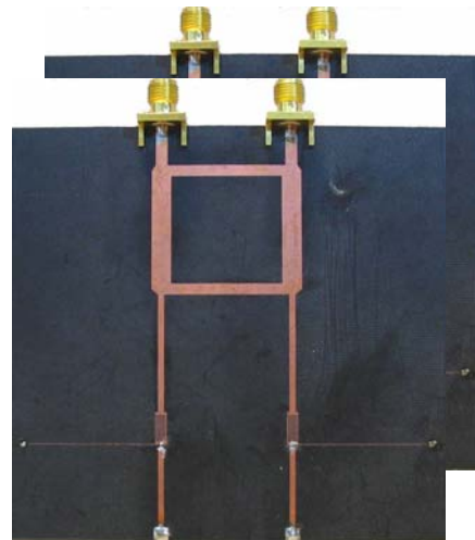
Figure 4: Prototype of a single-resonator microstrip Bandstop Limiter.
