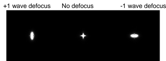
Figure 3b: In focus and phase diverse point spread functions with 1 wave of astigmatism. The phase diverse PSFs are different.
