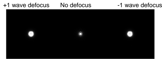
Figure 3a: In focus and phase diverse point spread functions for no aberration. The phase diverse PSFs are identical.
