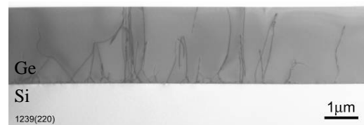
Figure 2: Cross section transmission electron microscopy (XTEM) image of germanium on silicon showing dislocations.
