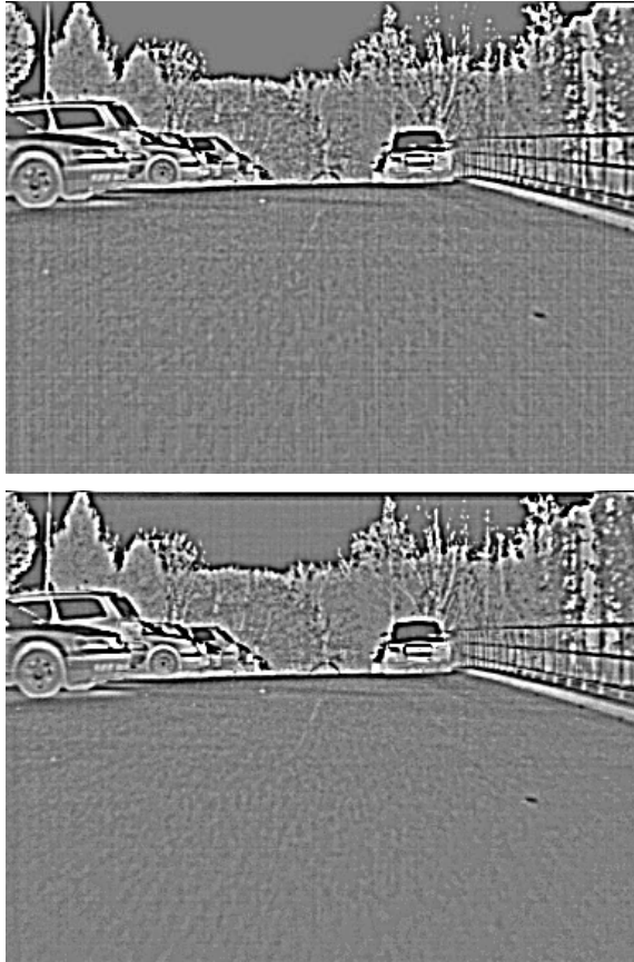
Figure 2: Typical IR images before and after FPN reduction (images are shown hi-pass filtered to enhance the noise pattern)
