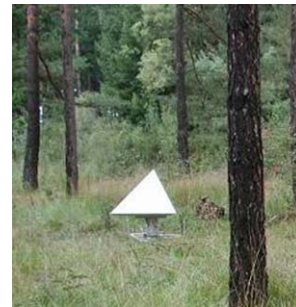
Figure 6. One of the 70cm corner reflectors placed under the forest canopy.
