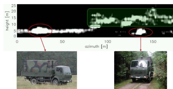
Figure 1. SAR Tomography allows a 3-dimensional picture of a scattering volume to be constructed in contrast to the usual 2-dimensional SAR image. The image shows two military trucks; one situated in a forest and the other in a field. The tomogram is clearly able to identify the truck despite the foliage which can be seen above it.
