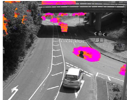
Figure 1 – Result of applying temporal differencing to vehicle sequence. Blue components indicate output of the detection, orange components are the accepted clusters (after morphology) and the pink components are the overlap of the two.
