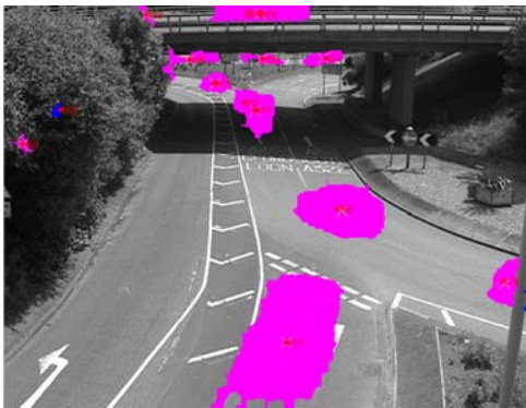
Figure 3 – Result of applying background subtraction to vehicle sequence. Pink components are the output of the detection.
