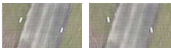
Figure 2. Motion blur significantly changes the appearance of objects; for example, this white object should be circular.
